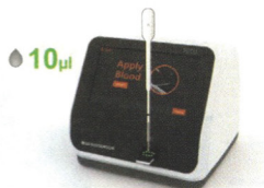
Add the 10µl of specimen into the specimen well.
