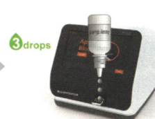
Add 3 drops of assay diluent into the assay diluent well.
